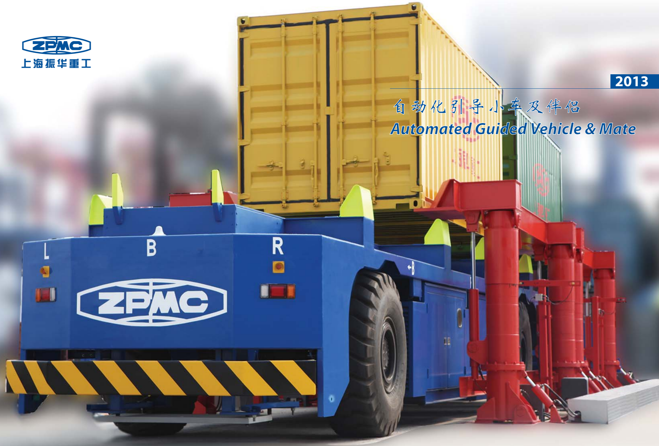
AGV驶入AGV伴侣以装载集装箱 AGV is going into the AGV mate to be carried containers
