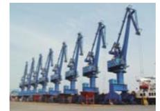
码头装卸门机 Terminal Bulk Cargo Handling Portal Crane
